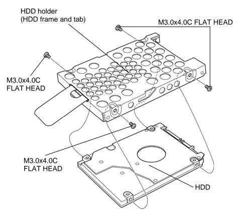
Figure 4-8 Removing the HDD
